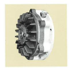
The disc type motor brake controls hook drift and facilitates load spotting. This spring-engaged brake is designed to operate if the air supply is interrupted for any reason. The motor brake is self-adjusting and incorporates cooling fins to dissipate heat. It is enclosed against dirt, water, and oil and is designed to independently hold the full rated capacity of the hoist.
