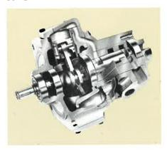
The Yale Cable King uses a heavy duty rotary piston air motor designed for high torque hoist duty. The motor provides excellent speed control for precision load spotting. It is lubricated by a continuous oil bath and incorporates an integral oil baffle, oil thrower, and large diameter crankcase breather plug. Normal operating air pressure is 90 psi. The four piston design provides for instant starting torque. Mufflers are standard.
