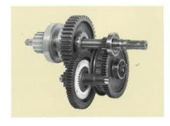
Gears and pinions in the Yale Cable King are machined from steel, and then case hardened to reduce wear. Gear teeth are full depth, 20 degree straight spurs with modified involute form. The full depth and involute design reduce strain and wear by allowing greater surface area contact. Each component is tested for hardness, accuracy, form and fit to exacting tolerances. The entire gear train is enclosed in a rugged casing and lubricated in a continuous oil bath.
